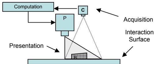
**Figure 1:** Set-up consists of key-stoned projector P, camera C and interaction blocks B
