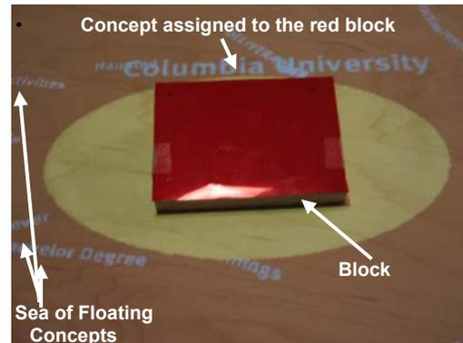
**Figure 2:** Blocks are assigned a concept and illuminated with a spotlight whose size and color is proportional to the importance of the concept assigned to the blocks
